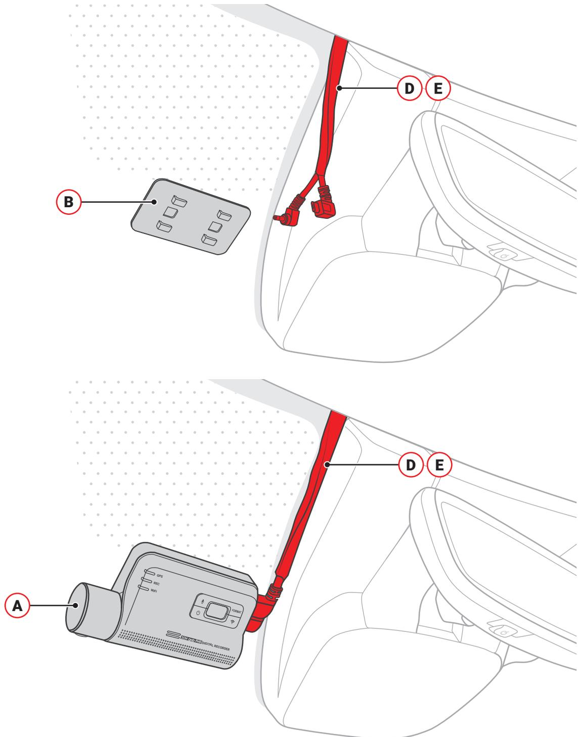
Proceed to Camera Connection instructions to “Live-View” the cameras and ensure correct orientation and visibility. Once confirmed, affix Front Camera (A) to vehicle with Front camera mount (B) and secure rear camera (C) to the rear windshield using the supplied and attached mounting tape.
