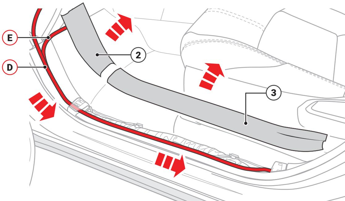
Prepare the cable path for **(D) + (E)** by removing the plastic door sill trims located at the edge of the interior floor. Hardwire Cable **(E)** can be left on the passenger floor area until the power is connected (Page 2).
