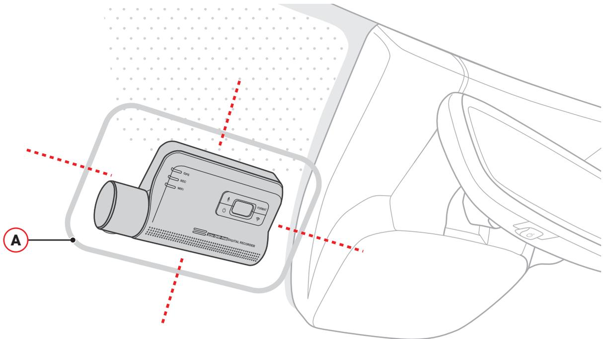
Insert Micro SD card (F) into the Front Camera (A) and connect power and video cables (D) + (E), Reconnect 12V negative terminal and re-fit all removed parts as per the vehicle workshop manual and Insert Micro SD card (F) into the Front Camera (A) and connect power and video cables (D) + (E).
