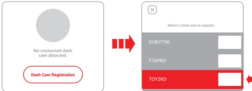
5. Hold the **Wi-Fi** button on the dash cam for 3 seconds, when the Wi-Fi LED starts blinking, tap the **'Bluetooth Connection'** button on your smartphone.
