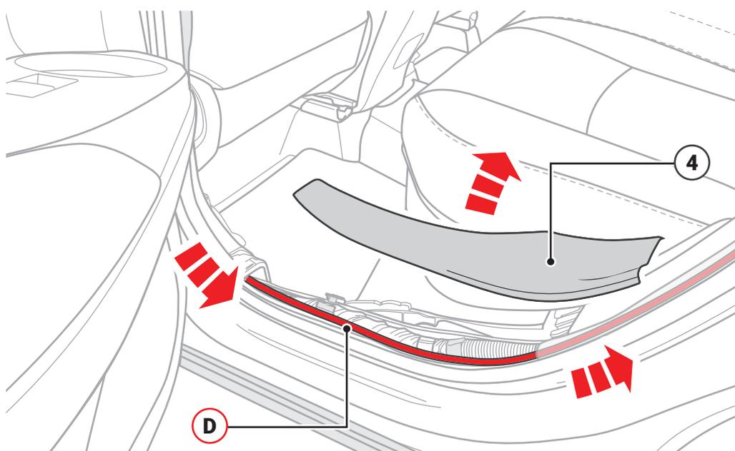
Follow path under rear scuff plate (4) and then under luggage compartment trim (5) when removed up towards headliner following OEM cable management where possible.
